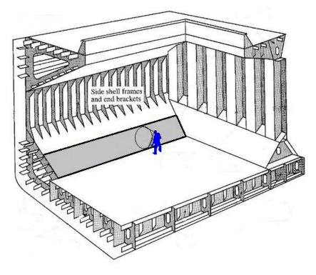
The previous figure shows the relative dimensions of a man in a cargo hold of a single skin capesize bulkcarrier and the shaded surface highlights the area that
